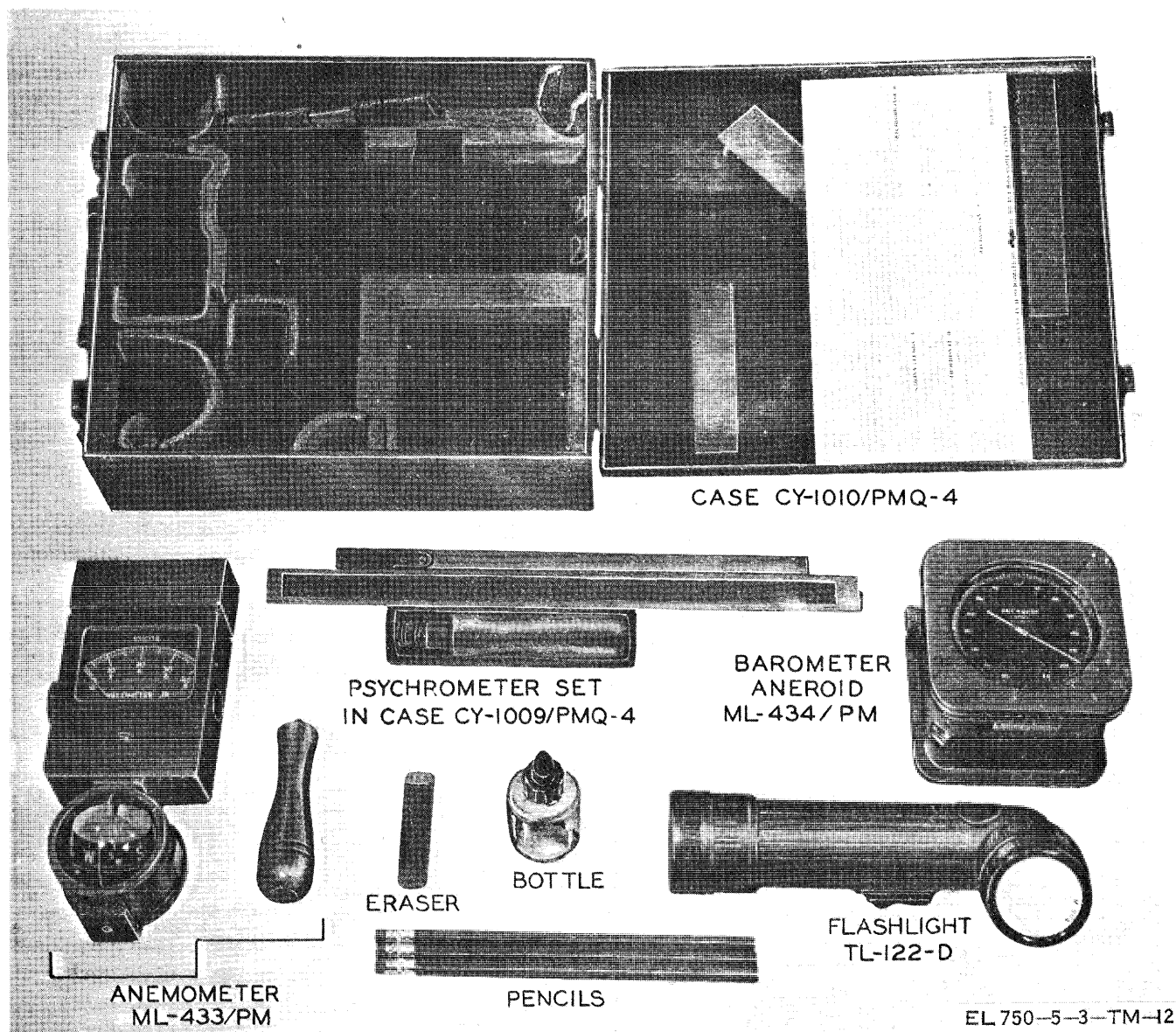
Figure 12. Meteorological Station, Manual AN/PMQ-4.
